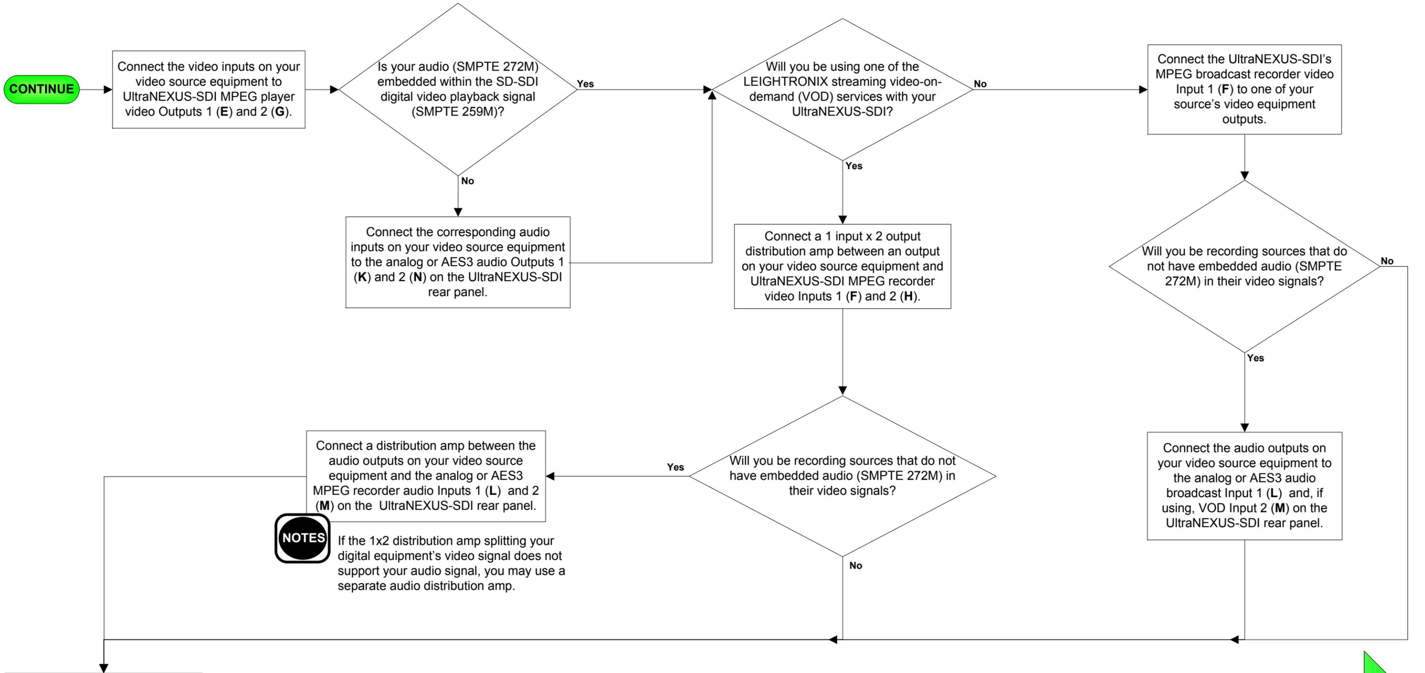
**NOTES** If the 1x2 distribution amp splitting your digital equipment's video signal does not support your audio signal, you may use a separate audio distribution amp.
